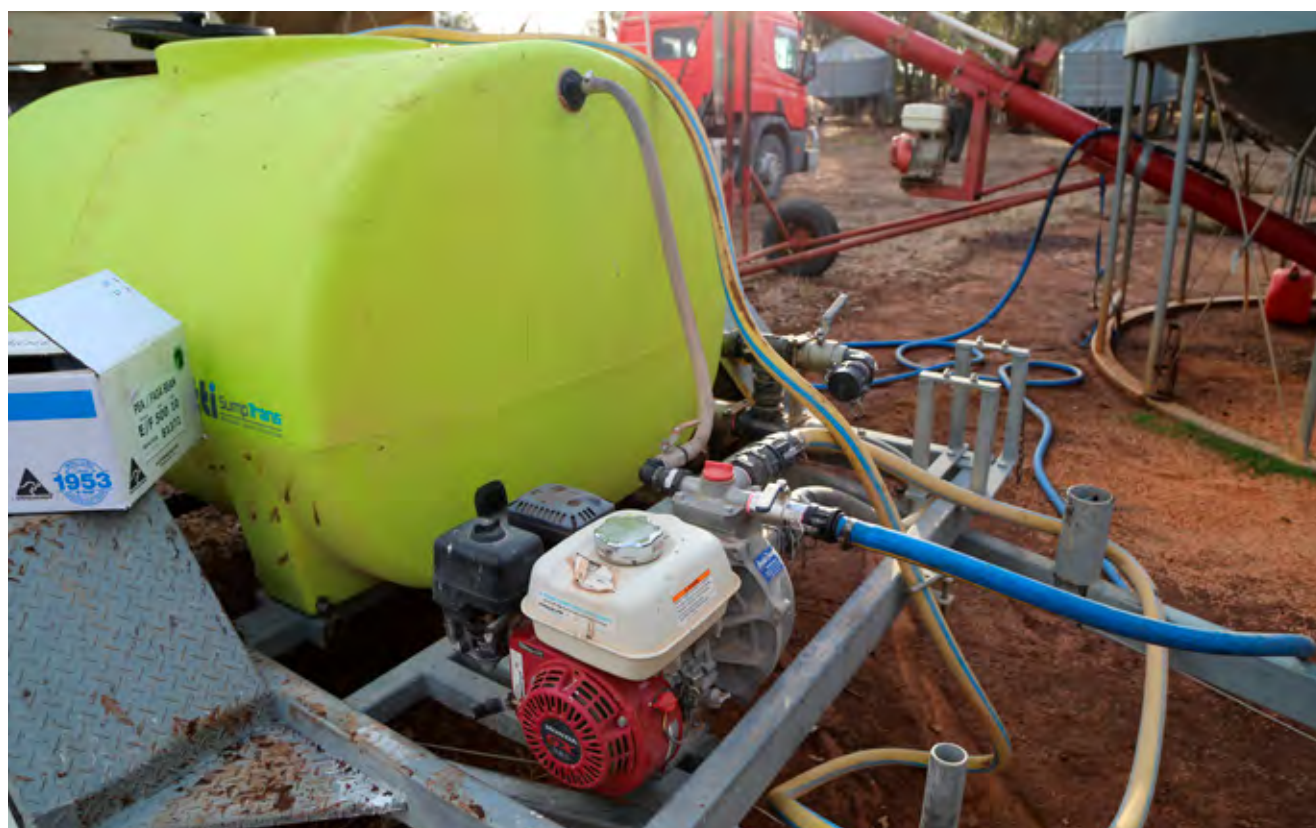
FIGURE 2-9 (b). Peat is added to clean water in clean spray tank where mixing occurs, pump allows for easy and adjustable flow to seed.
