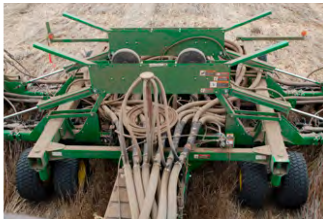
FIGURE 2-14 (d). For this air-seeder the seed, fertiliser and granules are mixed together in the air flow just prior to delivery to the soil furrow.
