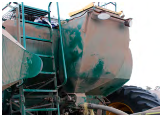
FIGURE 2-14 (d). For this air-seeder the seed, fertiliser and granules are mixed together in the air flow just prior to delivery to the soil furrow.
