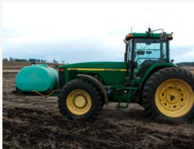
FIGURE 2-13 (b). Water tank mounted on tractor to apply inoculants by water injection.
