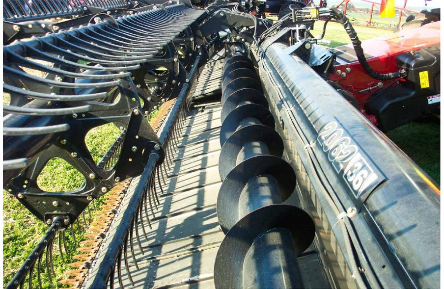
**Photo 1:** Belt-front fitted with cross-auger.
