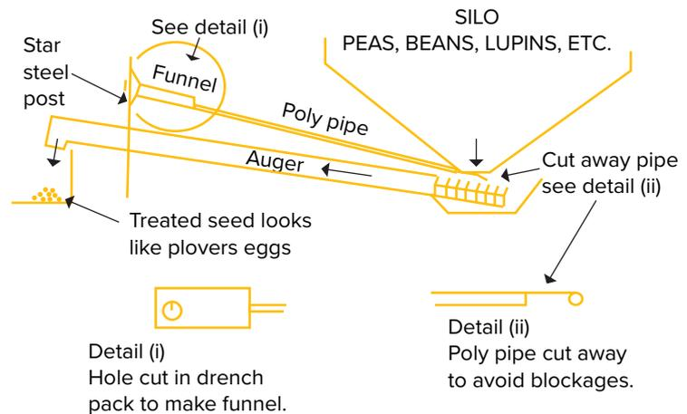
**Figure 2:** Applying inoculum through an auger.
