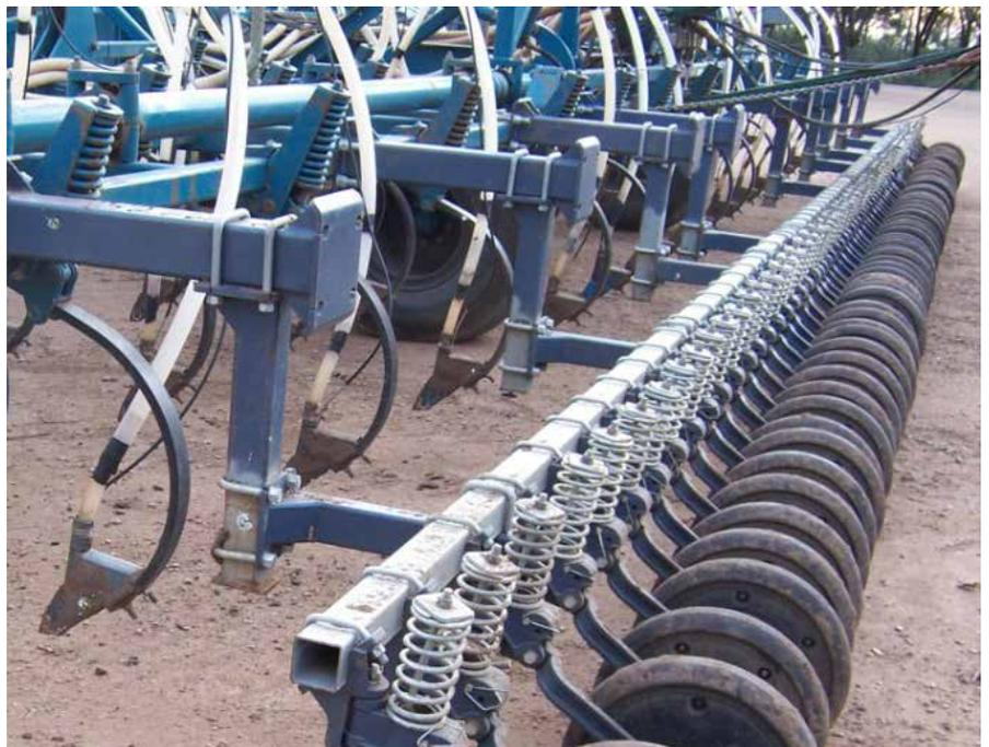
**Photo 5:** *A seeding bar setup with Atom Jet narrow points, gang press-wheels and liquid injection for either inoculum or trace element application during sowing.*
